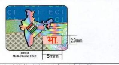
4 Motion Effect takes place in the blue background where the letters ECI move horizontally out and in simultaneously giving a wavy effect.
